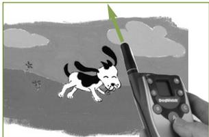
How you hold the transmitter may affect the range. For maximum range, keep the antenna pointed toward the sky. *Pointing the transmitter antenna toward your pet will reduce the range.*
