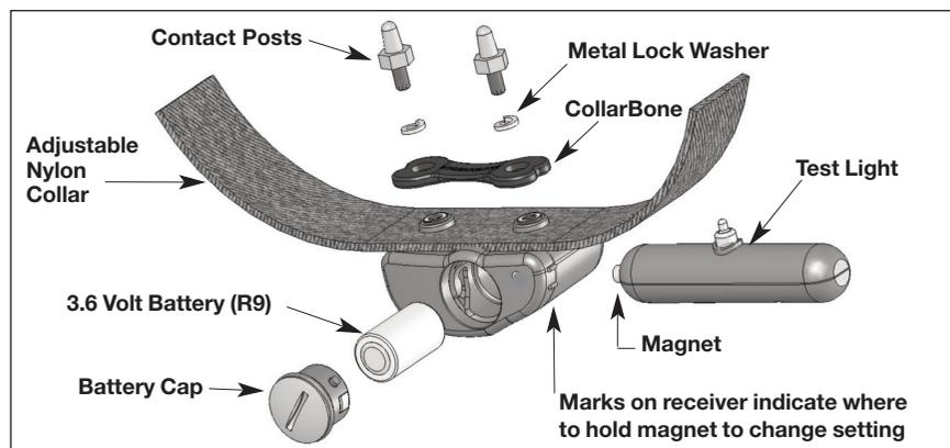
The components of both the R9 (above) and the R7m are the same except the R7m is smaller and uses a different battery.
