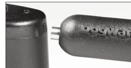
Using the magnet to reset the R9.
